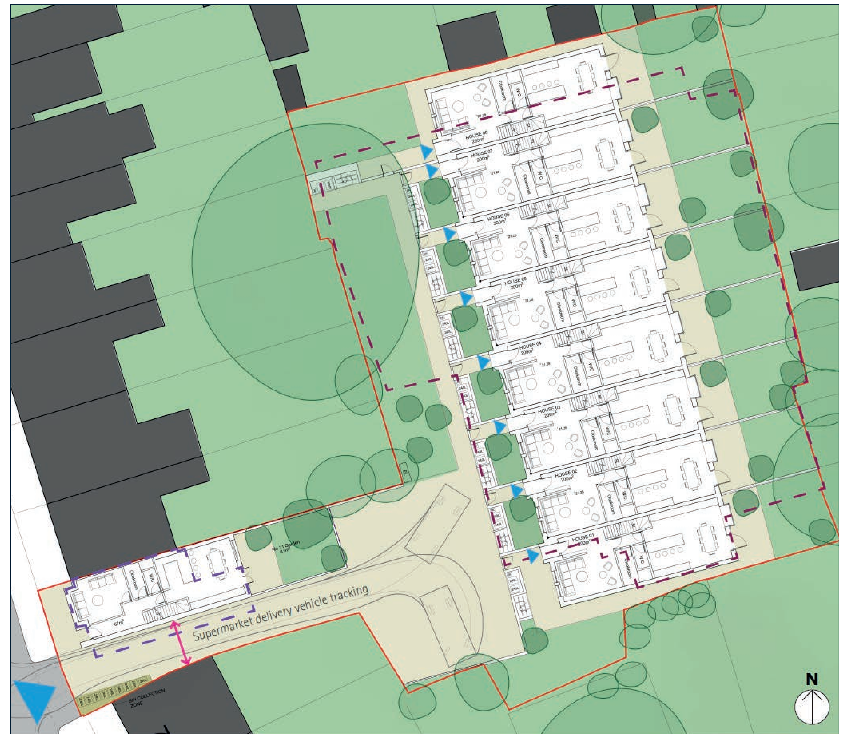
Indicative Ground Floor Layout: Proposed Plans Overlaid on Existing Building Line (Denoted by Grey Dotted Line)
